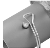
Fig 3 Improperly Secured Leg Coupling Pin
